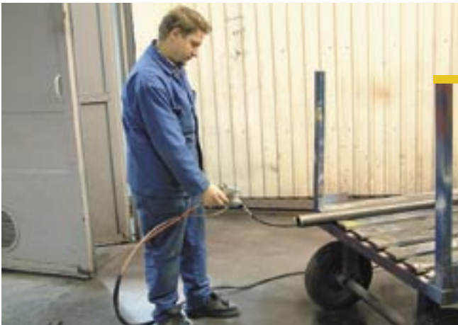
Prior to shipping the pipe end is carefully plugged.
