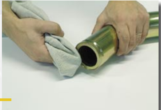
The dowty seal is greased before installation.
