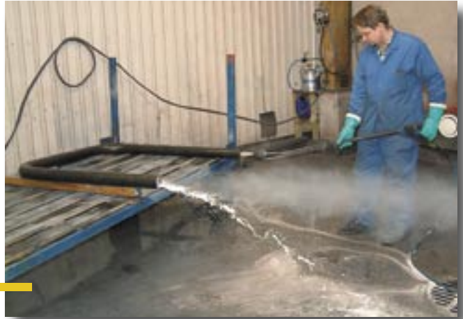
Piping modules are protected with oil in order to prevent corrosion during transportation and storing.
