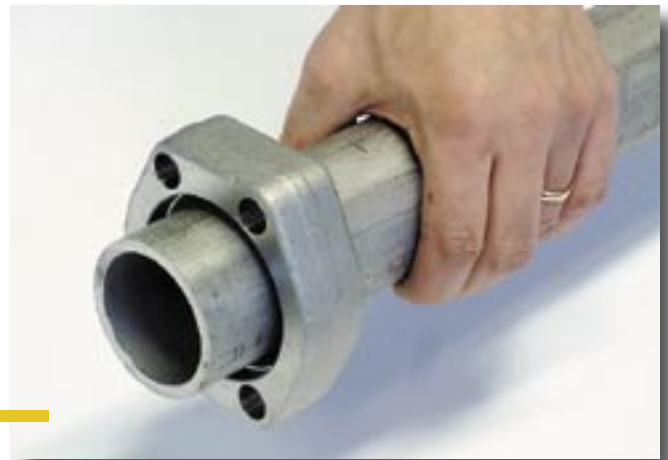
Prior to flaring the dye and the flaring cone is cleaned. Oil is used on the flaring cone and on the pipe end.
