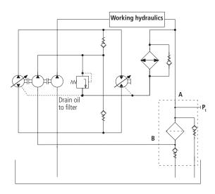
The entire dirt produced in the hydrostatic drive by abrasion is filtered out immediately and is thus not taken in by the pump of the open-loop circuit. This circuit layout is always recommended if the return flow only slightly exceeds the suction flow, i.e. if there is
