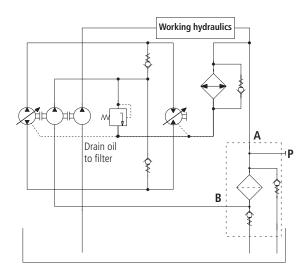
The entire dirt produced in the hydrostatic drive by abrasion is filtered out immediately and is thus not taken in by the pump of the open-loop circuit.
