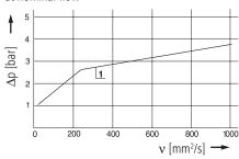
Pressure drop as a function of the **flow volume** at  $v = 35 \text{ mm}^2/\text{s}$  (00/01 = casing empty without/with hole Ø 4 mm)
