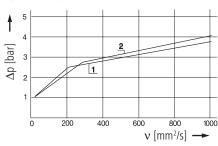
Pressure drop as a function of the **flow volume** at v = 35 mm<sup>2</sup>/s (0 = casing empty with hole Ø 4 mm)
