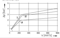
Pressure drop as a function of the flow volume D<sub>2</sub> at  $v = 35 \text{ mm}^2/\text{s}$  (0 = casing empty)
